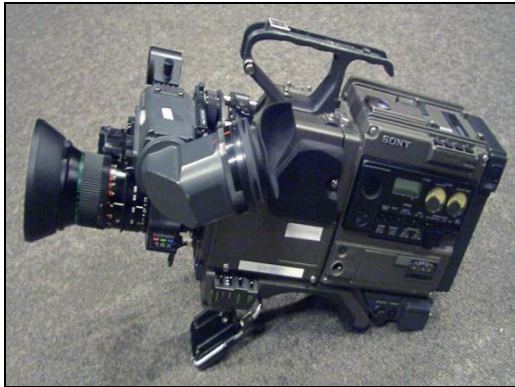
Fig 2: Example of ENG (electronic news gathering) video camera
